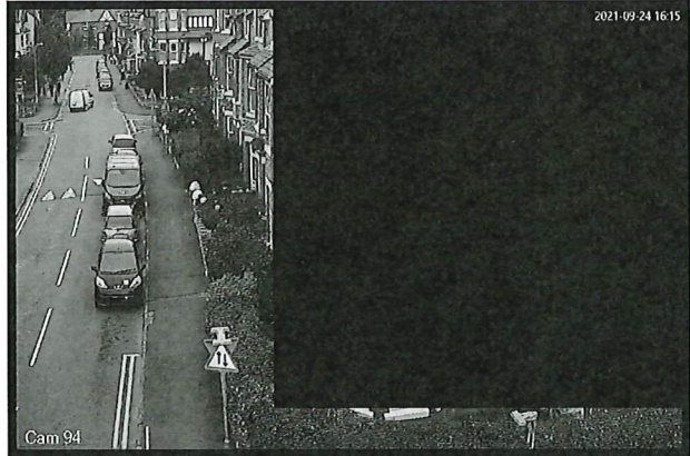
Figure 2; Actual privacy zone on a current camera view
